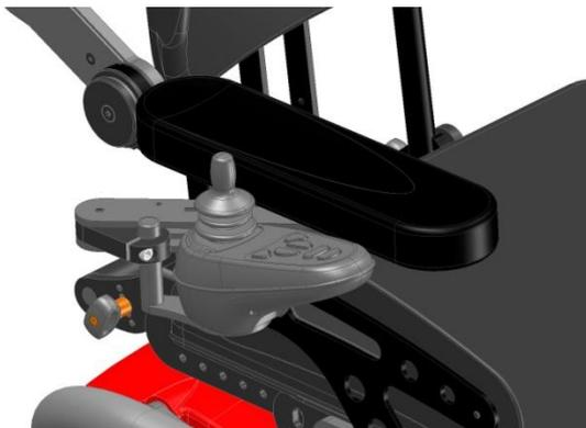
The swing away joystick holder is used to drive closer to a table for example. The transfer can also be easier, if the control unit is retractable.
