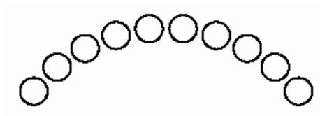
The battery gauge shows you that the wheelchair is switched on and it shows you how much power there is left in the batteries. The gauge is also used as an electronic fault detection (see chapter 16.)
