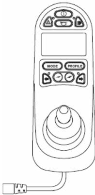
On the control unit you can find a joystick, buttons and a LCD-display, where we take a closer look at in the following.
