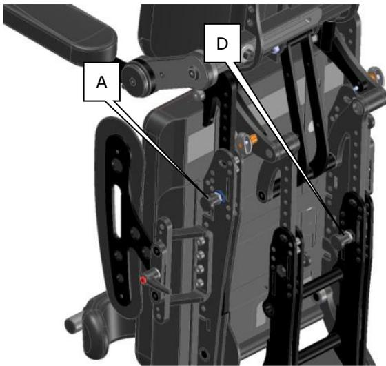
The seat depth will be adjusted with (optional w/o) tools. Adjust the lower levers first. Release the screw (pull the bolt) (C) and (D). Now you can set the levers to the necessary length. Tighten the screw (release the bolt) and lock the lever in the new position.
