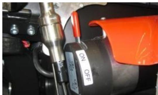
To disengage the motor brakes, to push the chair manually, switch off the control, pull the quick release knob (A) and press the lever (B) down respectively the lever from ON to OFF
