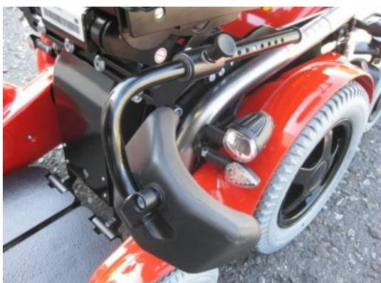
There is also a park position which provides to stay the knee support Integral in place by any transfer.
