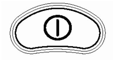
With the On-/ Off-button the chair can be turned on or switched off. Don't use this button to stop the wheelchair, unless there is an emergency.
