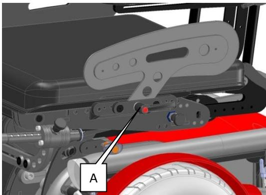
The skirt guard should prevent that the clothing is hanging beside the seat and is getting into the drive wheels or the standing mechanism. The skirt guard is easily displaceable for lateral transfers. Just untighten the stop lever (A), now you can easily lift the skirt guard upwards to remove it.
