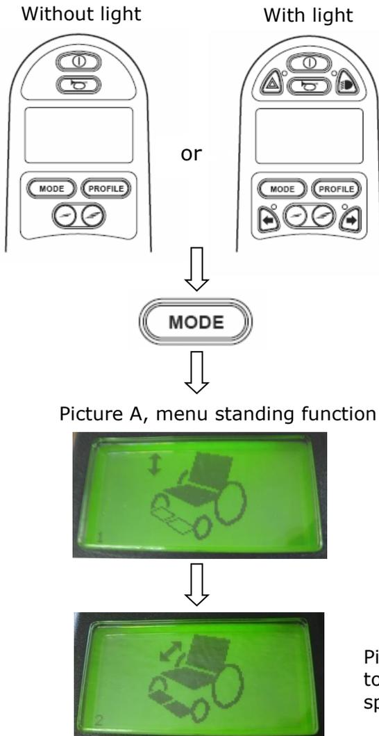
By pressing the MODE-button, you get into the standing function menu (picture A should appear on the display). If you now press the joystick forward, the seat is raising, if you press the joystick backwards, the seat is lowering.
