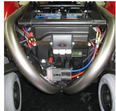
Open the fuse cover, insert the fuse which is delivered in a separate plastic bag and snap the fuse cover back. Now the chair can be brought into standing position to get access to the fuse cabling. Store the fuse cabling properly above the batteries and the main fuse housing below the control system under the chairs cover.
